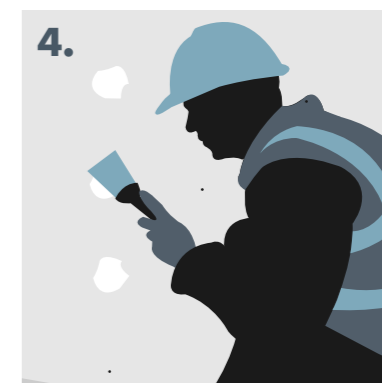
Covering screw heads with Knauf Aquapanel Exterior Joint Filler - Grey.
