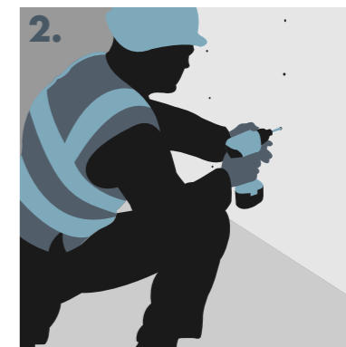
Fixing the boards to the background members.
