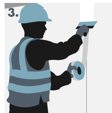
Embedding Knauf Aquapanel Exterior Joint Tape.
