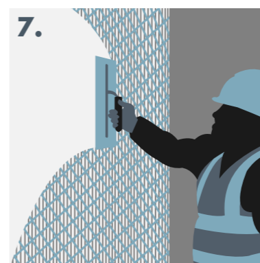
Covering mesh with basecoat.
