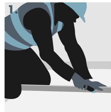
Scoring Knauf Aquapanel Exterior Cement Board with a knife.
